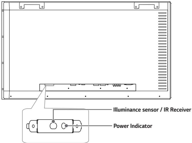
**Illuminance sensor:** Adjusts the screen brightness by measuring the amount of light.
