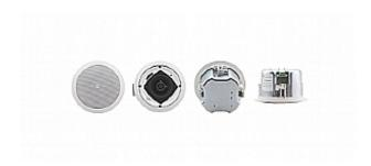
The Galil 4–C Closed-back Compact Ceiling Speaker features a multi-tap power transformer for selecting  $8\Omega$  (bypassing the transformer) or 70V/100V power settings that are suitable for an array installation. The Galil 4–CO open-back version is also available.
