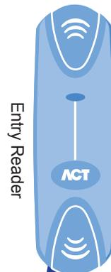
For Clock & Data Readers, wire exit reader in parallel but leave it's sense line unconnected.
