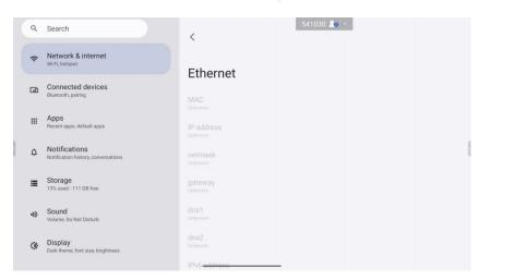
In automatic configuration, the system automatically obtains the IP address and other information about the Ethernet and establishes the connection. In manual configuration, you need to manually enter the corresponding information. Ethernet proxy can be configured for proxy-based access.
