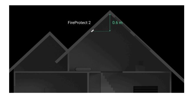
We do not recommend mounting the detector on a wall. This installation is acceptable if closely spaced beams or other obstacles interfere with the installation of the detector. Wall mounting is possible only if the detector
