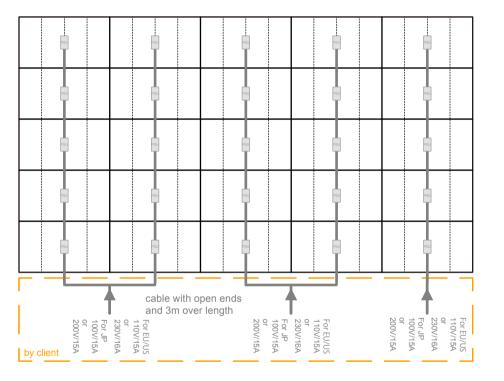
The 15A(US) or 16A (EU) circuit breaker for the each power feed must have a european D characteristic or similar. (can hold for a short term 20times the tripping current)
