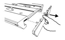
Examine the illustration below and proceed with the removal of the spring pin(2). Remove from holes in two steps:
