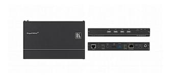
The TP-590RXR is a high-performance, extended range, HDBaseT 2.0 receiver for HDMI, USB 2.0, audio, bidirectional RS-232 and IR signals. The TP-590RXR receives the HDBT twisted pair signal from the TP-590TXR that it decodes back into HDMI, USB, audio, RS-232, and IR signals.
