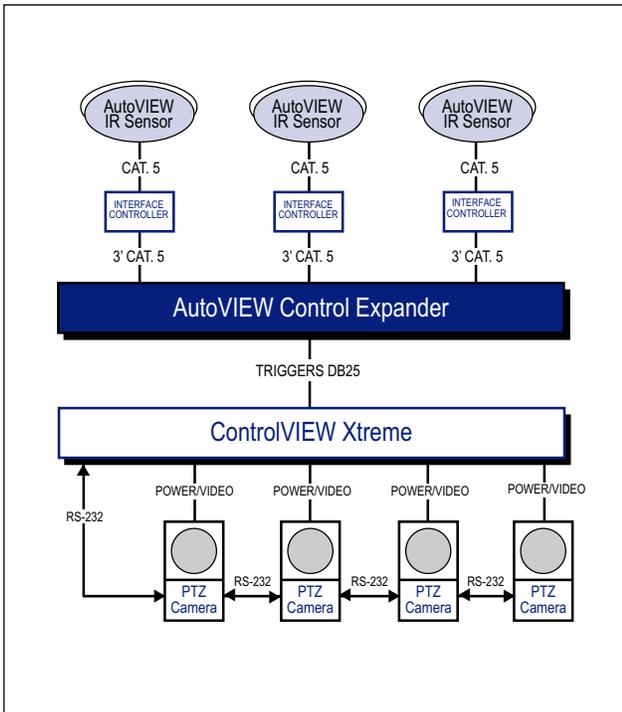
Figure 2 – Three sensor AutoVIEW IR System.
