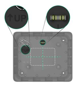
2. Prepare cable entries in advance: drill holes for cable glands on the bottom, top, or sides of the casing, or break out the perforated part on the back of GlandBox. We recommend using a Ø20 mm hole saw for plastic.
